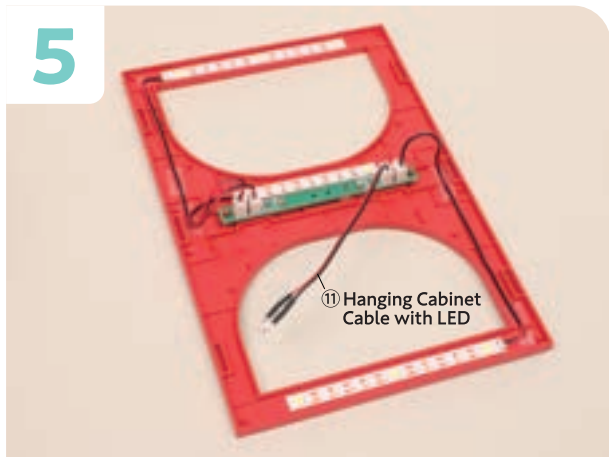
Plug the connector of the ⑪ Hanging Cabinet Cable with LED into the remaining socket on the Circuit Board.
